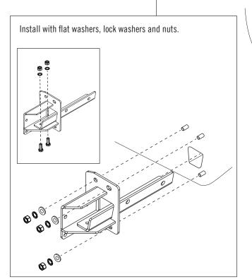
On the underside of the vehicle, fix the brackt in place using M8 toothed and flat washers and M8 hex bolts.
