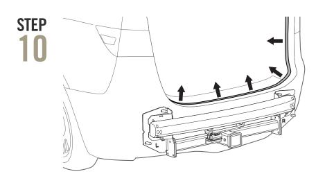
Carefully lift off rubber lining.
