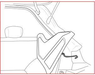
Splice the trailer plug wiring directly into the tail light wiring. There is no need for an ECU.
