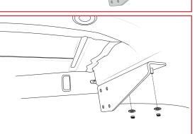
Using a large washer and nut, finger tighten the brackets in place.
