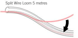
Route wire with Split Wire loom to battery terminal. Secure with Zip-ties
